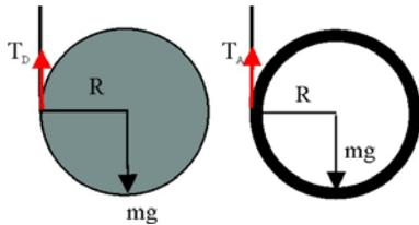
$$mg - T_D = ma_{CMDisco}; \quad R T_D = I_D \alpha_D; \quad R T_D = \frac{mR^2}{2} \alpha_D; \quad T_D = \frac{mR}{2} \alpha_D = \frac{ma_{CMdisco}}{2}$$
