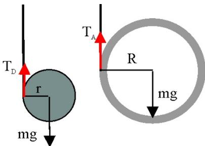
$$mg - T_D = ma_{CMDisco}; \quad r T_D = I_D \alpha_D; \quad r T_D = \frac{mr^2}{2} \alpha_D; \quad T_D = \frac{mr}{2} \alpha_D = \frac{ma_{CMdisco}}{2}$$
